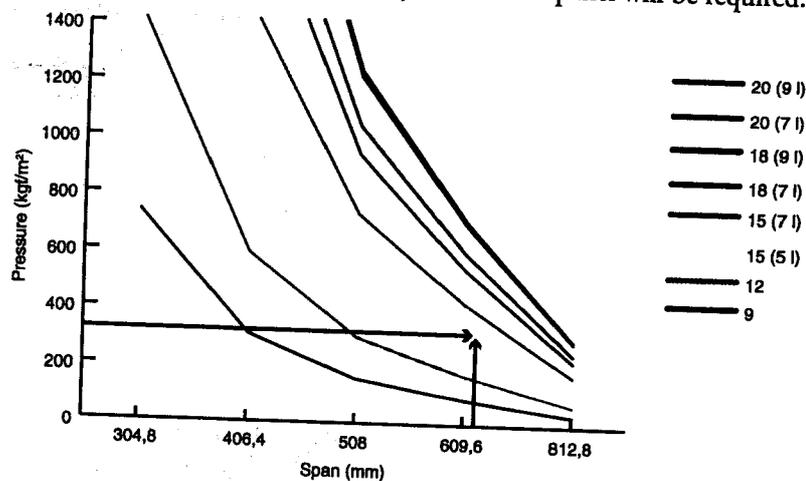
Figure 06 – Determination of the minimal plywood thickness.
